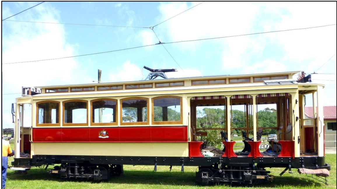
Tram 17 on its first test tow on its Brill 22E trucks, 27 th November 2019.
