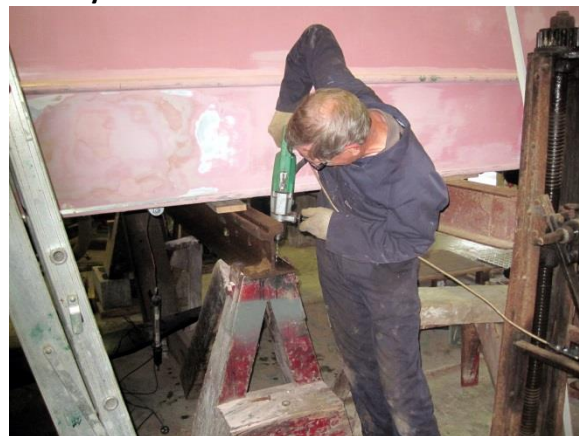
(1) Above: The large transverse lifting beams had to be extracted from under tram 260. They were replaced with sections of tram rail. Here Colin Dash is drilling a hole in the base of the replacement tram rail section to enable it to be securely fastened to the side supports. One of the large tram body jacks can be seen, with the attached lifting beam supporting the tram.
