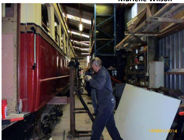
(5) Above: After lifting the tram sufficiently with small jacks to enable insertion of the large lifting beams, (and after lunch!) the main lifting commences. Someone on each of the four jacks and unified lifting to keep the tram level. Marlene Wilson
