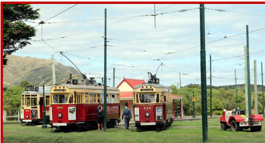
Left: The three service trams on 27 th January. Tram 239 on the right has stopped just short of the "still to be done" overhead on workshop road 5 and will be shunted into the workshop using the Clarktor tractor on the far right. Photo: Allan Neilson
