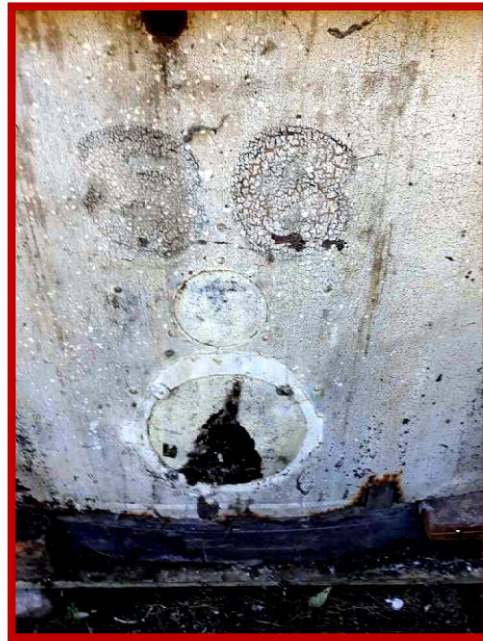
Above: Part of the "A" end apron of tram 86, showing the faded and disintegrating number, and the tail light and headlight area.
