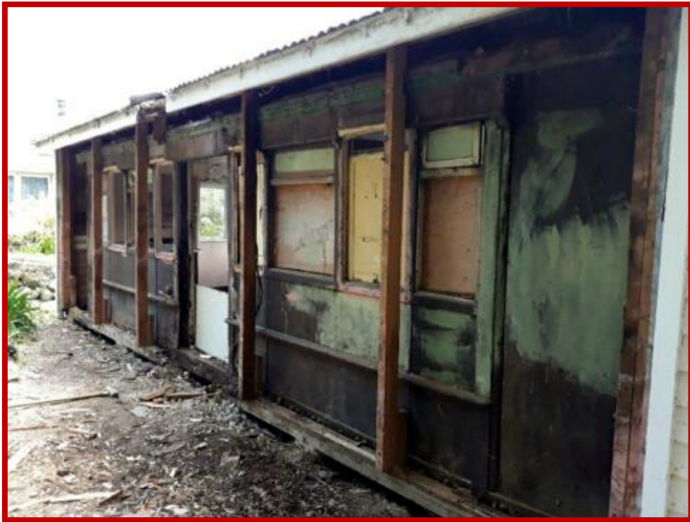
Above: This photo, taken on 14 th January prior to dismantling of the roof but following removal of the outside wall shows one side of tram 86 almost intact and still in its 1920's chocolate brown colour.
