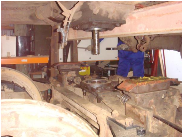
18 th June – carefully lowering tram 159's king pin into the bearing on the truck. Photo: Robert Hatten
