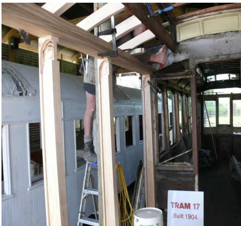
Above: New cant rail and pillars in place. 7th August
