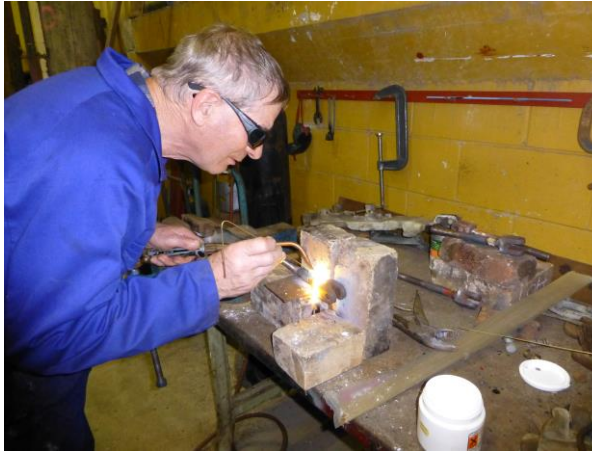
Colin Dash brazing a component for tram 260's magnetic brakes.
