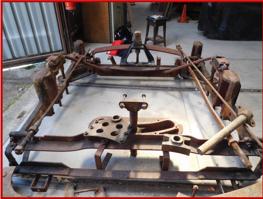
Above: The Brush Truck mocked up. Looking from the driving wheels end and illustrating the layout of a 22E Truck
