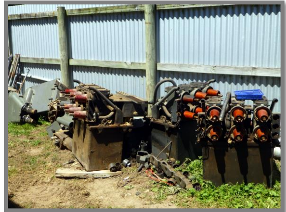
The removed 11KV switchgear has been placed in our storage compound for further dismantling and disposal.
