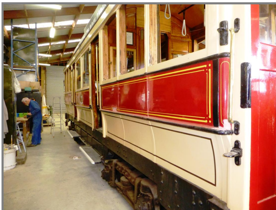
Above: Tram 159 is currently in the position in the workshop long occupied by tram 260. It is undergoing a general refurbishment. Note that the saloon windows have been removed. Photo: Keith McGavin
