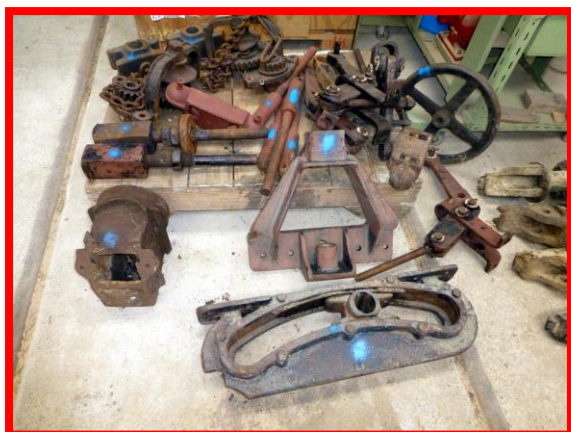
Above: Various tram truck parts, marked with blue paint, set aside for use in the reconstructed trucks for tram 17. Photo: Keith McGavin
