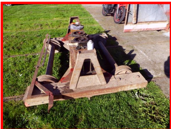
Above: Sammy truck being fitted with modifications – to go under tram 185 in the rear storage building.
