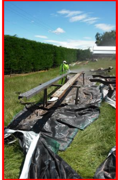
Above: Sandblasting of steel chassis
