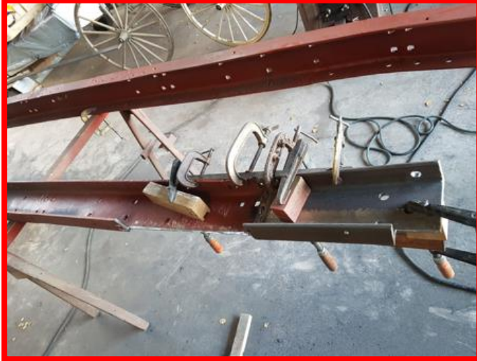
Above: New pieces being welded into the chassis to replace corroded areas
