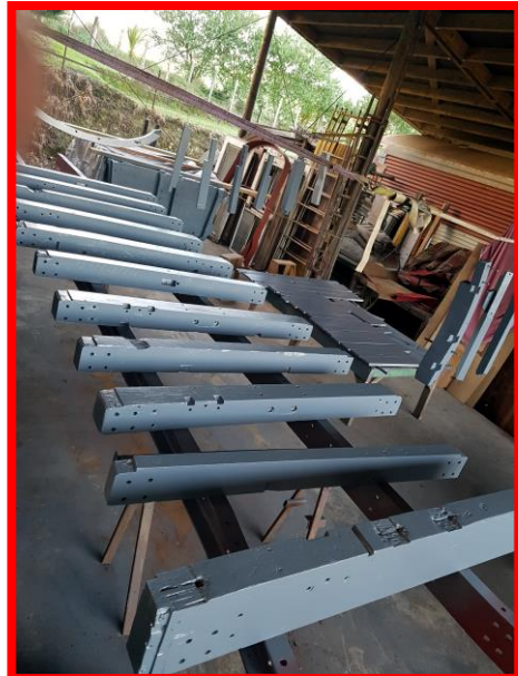
Above: Preparation and painting of timber chassis components
