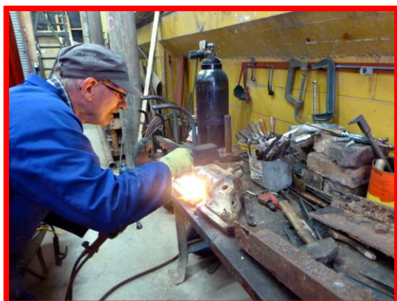
Above: Colin Dash removing the outer casing from a magnetic brake unit that will be rewound and renovated for use on tram 17, 7 th June 2017. Photo: Keith McGavin
