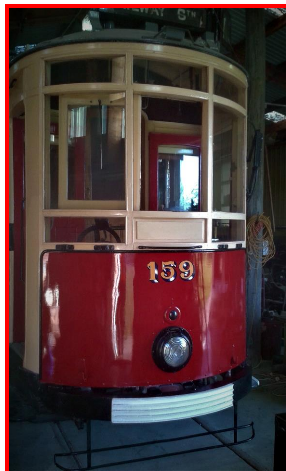
Above: Tram 159 in the workshop: The "A" end and apron repainted and with taillight and headlight refitted, 21 st June 2017. Photo: Russell Jenkins
