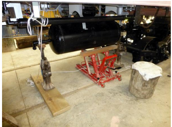
8. 23 rd September: Mounting the air tank.
