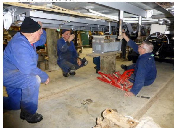
3. 2 nd September. Installing a resistance grid
