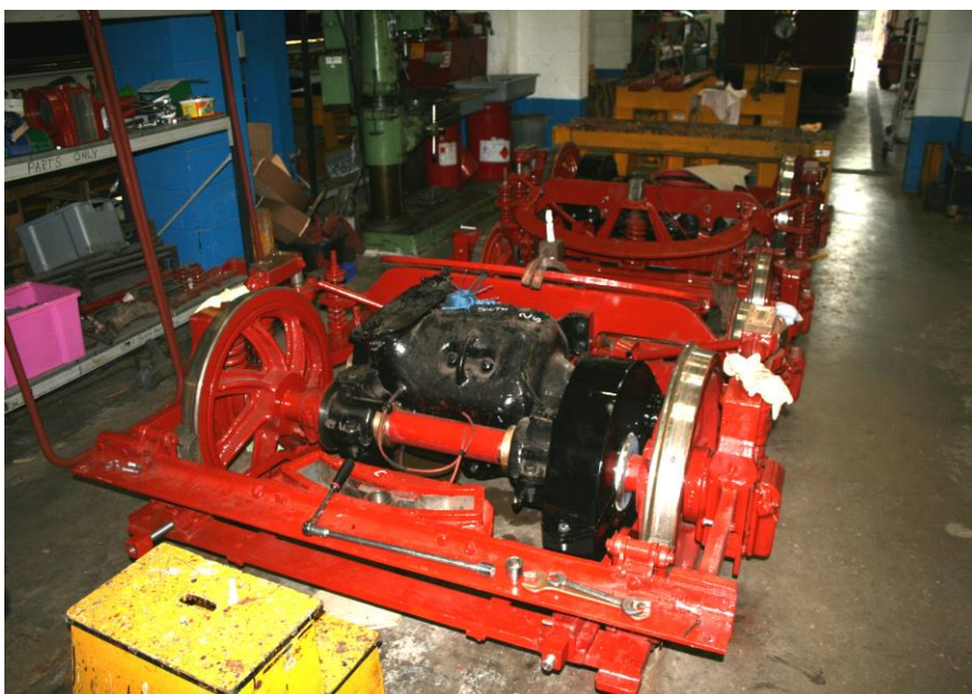
Above: Nearly completed 22E trucks for London United Tramways (LUT) No.159 at Crich, U.K. This illustrates what ours will look like once they are assembled.
