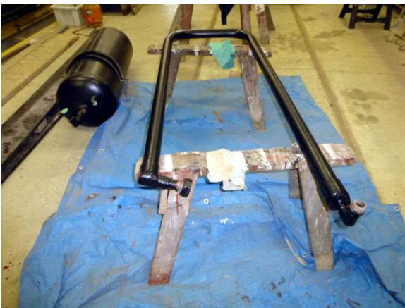
6. 16 th September. Preparing air tank & piping
