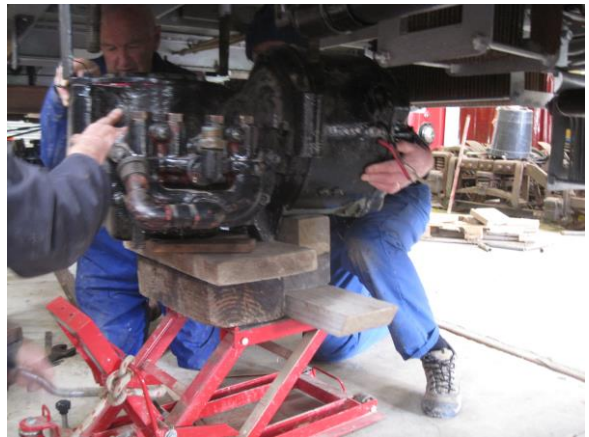
9. 7 th October: Mounting the air compressor.
