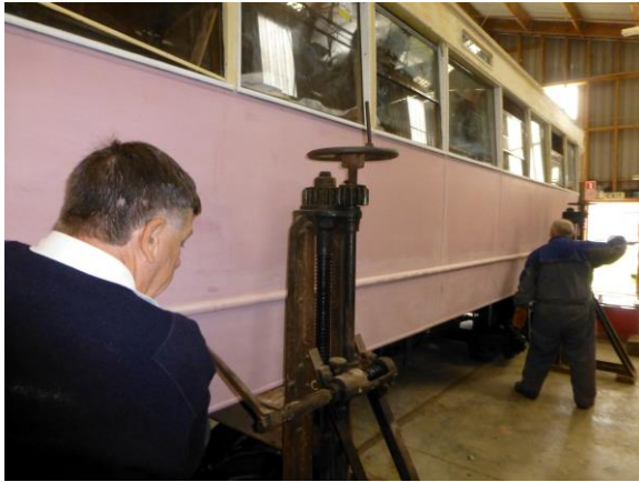
10. 14 th October: Lowering the tram on to its trucks. First time on wheels for several years!
