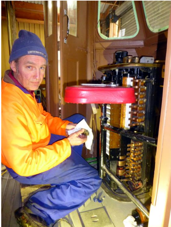
4. 2 nd September: Allan Neilson – electrical work on controller
