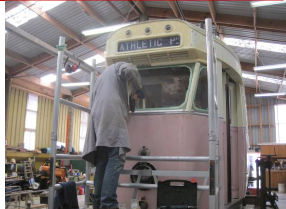
2. 2 nd September. New beading installation under windscreen.
