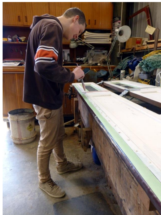
Above: Brendan Bulliff applying paint to one of the repaired folding doors for tram 260, 15 th October 2014.
