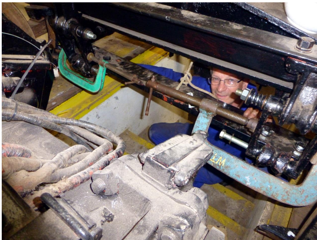
Above: Colin Dash is under there! The process of fixing the very heavy main brake beam in place on the A end truck for 260 - with the aid of G clamps and rope! 15 th October 2014. Photo: Keith McGavin
