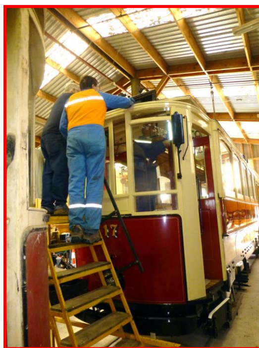
Above: Trevor Burling (left) and Grant Johnson on 29 th May 2019 test fitting mechanisms associated with the destination box on the roof of Tram 17 “B” end. Photo: Keith McGavin
