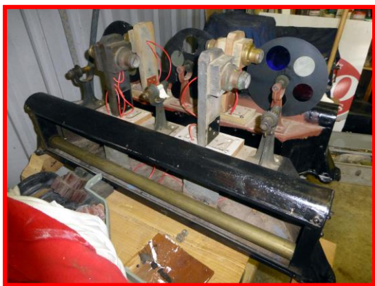
Above: One of the two destination box and coloured light mechanisms, dismantled into its component parts.
