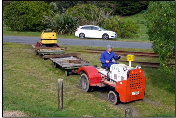
Above: Our rail lifting and moving equipment at the loop heading for the rail stack on 26 th August. It comprises the "Tug" tow-motor and two wharf trailers – plus the digger which is loaded on the rear trailer.
