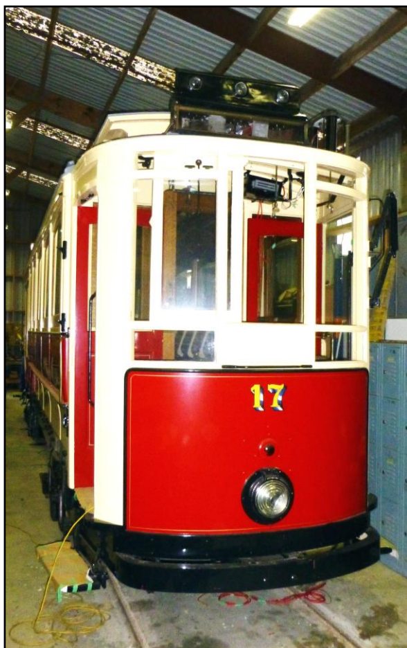
Above: Tram 17 in the workshop, from "B" end. Note destination/coloured light signals and number boxes in position. 19 th August 2020.
