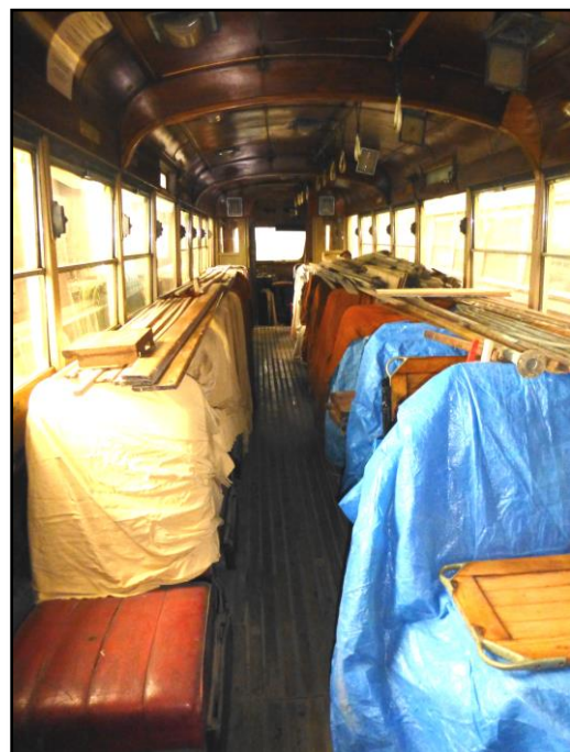
Above: The interior of out-of-use Fiducia tram 238 in which are stored many restored and unrestored parts from 207 including newly varnished timber panelling strips, plus the hinged timber seats and the seat frames from the centre saloon. 8 th July 2020.
