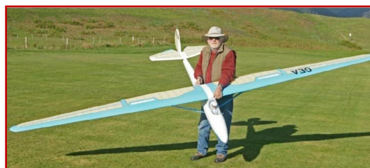
Above: 5 m span glider. 1/3 scale model of a Kirby Kite.
