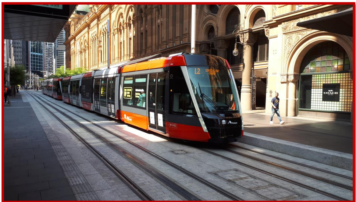
Sydney Light Rail Vehicle in George Street – Note the “3 rd rail” that provides power to the vehicle.
