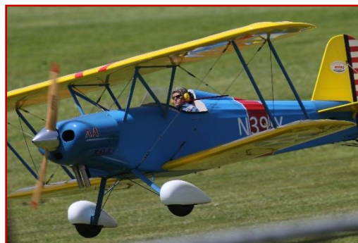
Above: Large scale biplane. 2,2m span. 80cc petrol engine
