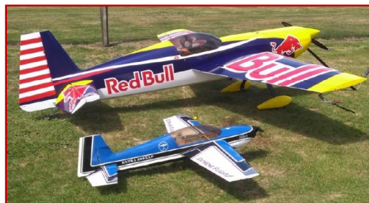
Above: 3.5 m 200cc powered Xtra and a 1200mm electric powered Xtra.
