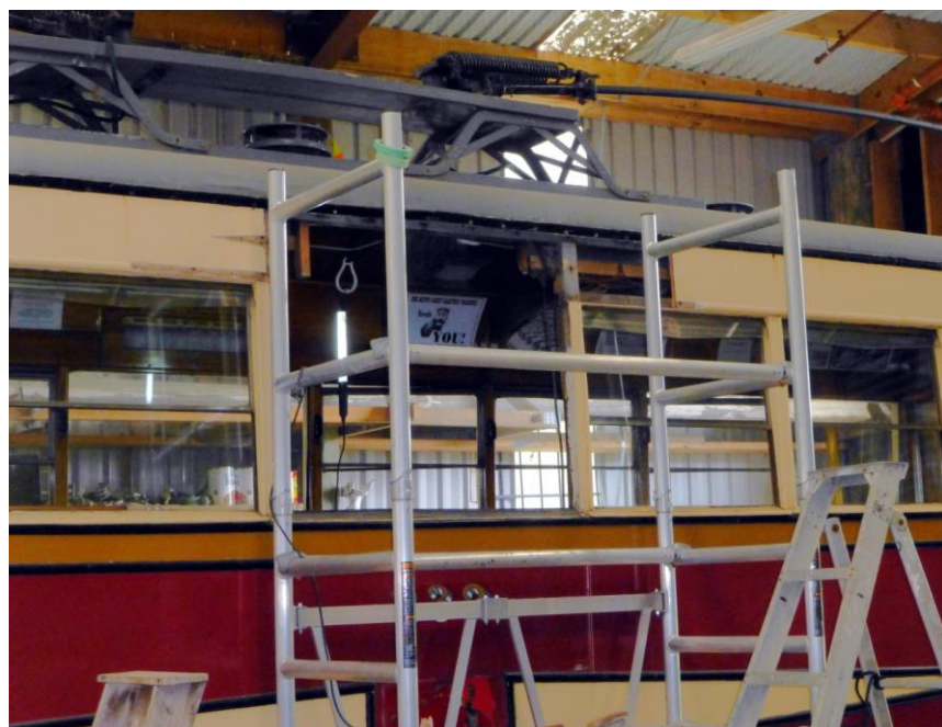
Above – results of the first day's work, 29 th April; window out, destination box and portion of letterboard around it removed.
