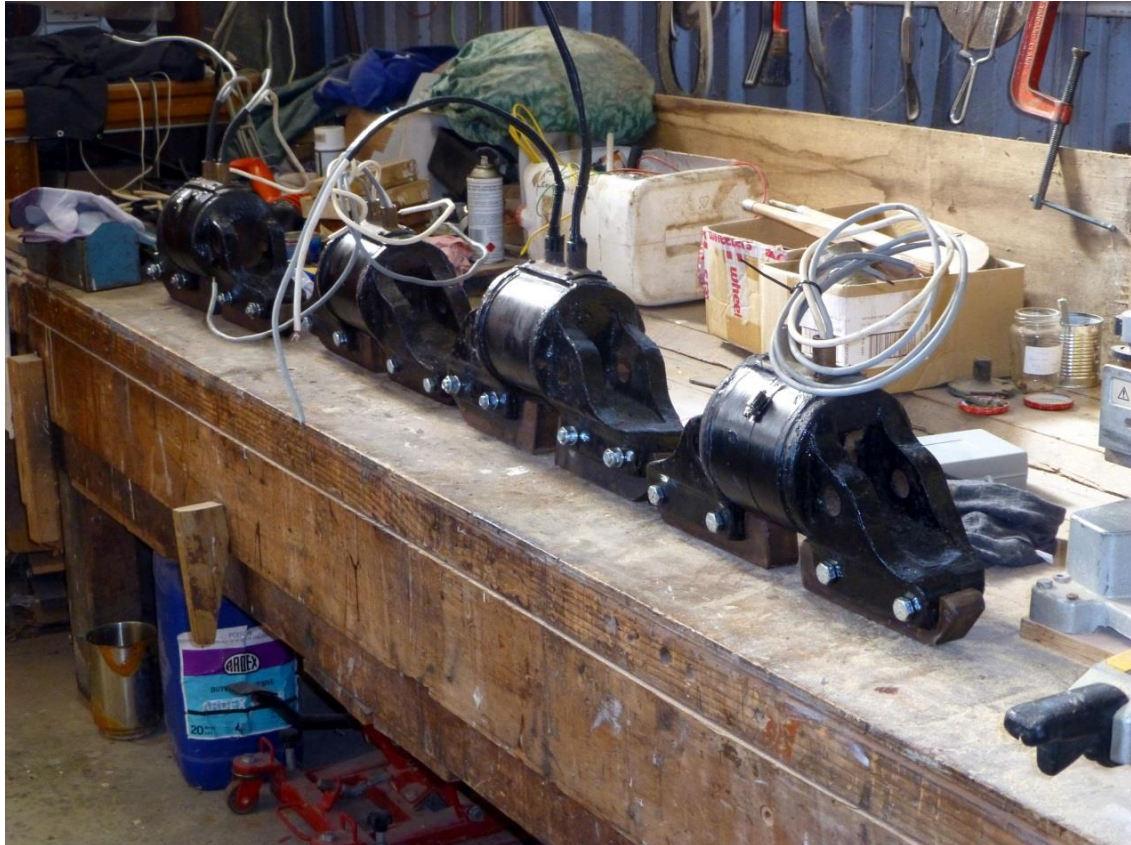
Above: Four rewind magnetic track brakes ready for 260, 25 th April 2015
