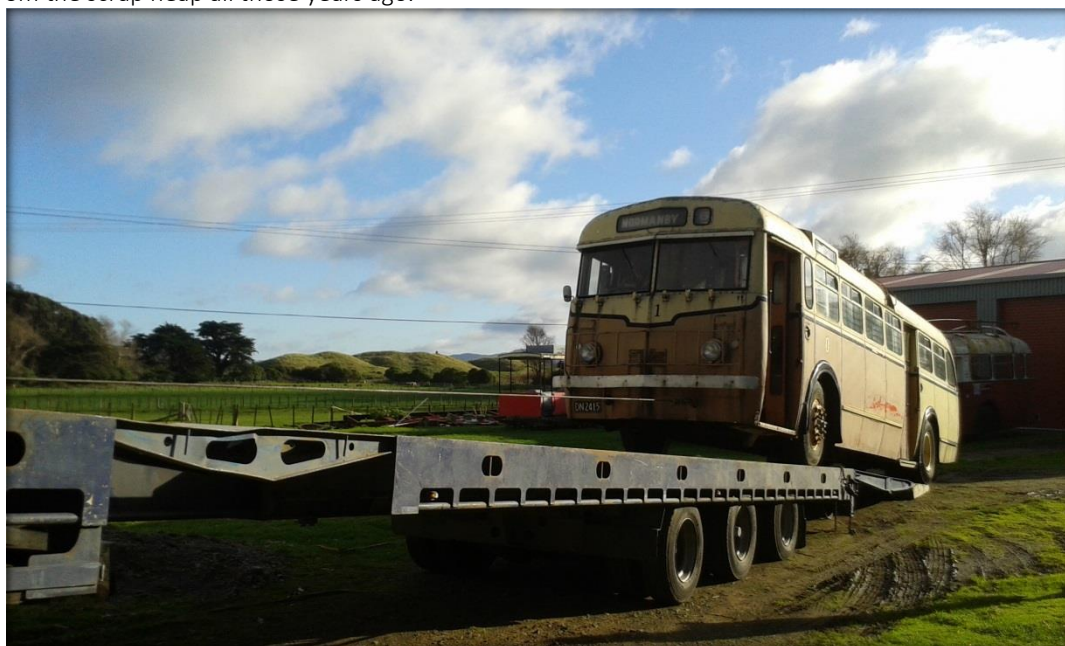
Above: Dunedin trolley bus No.1 is "driven" on to the low loader by the truck driver in the bus cab using a remote controlled winch, 26 th June 2015.
