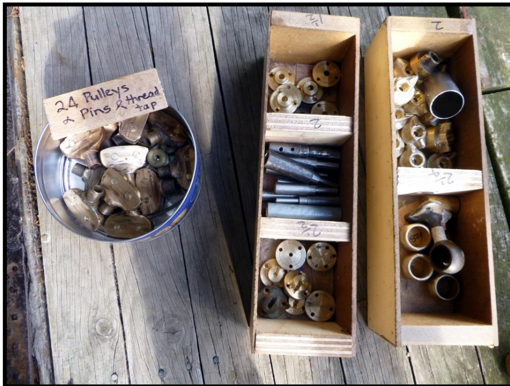
Above: New brass and other metal components have been manufactured for the blind mechanisms. The blind material is on order. Photo: Keith McGavin
