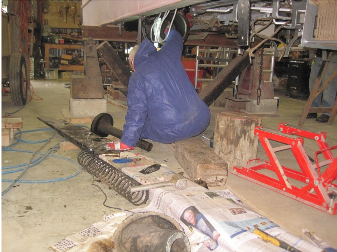
Above: 260 - The brake cylinder being dismantled to remedy an air leak, 6 th May. Photo: Mike Flinn
